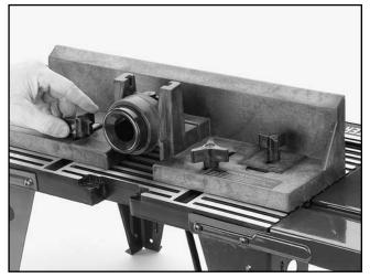
Figure 14. Securing the fence to the main table.
